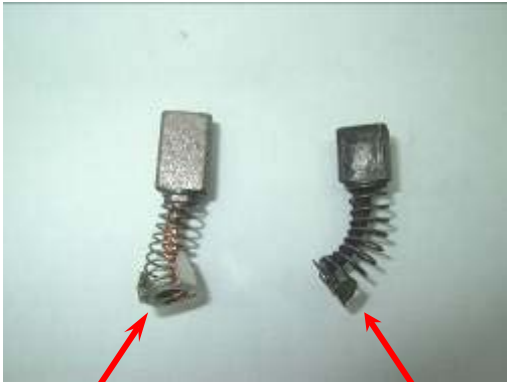
New Motor Brush Worn Motor Brush (Fig 41)
